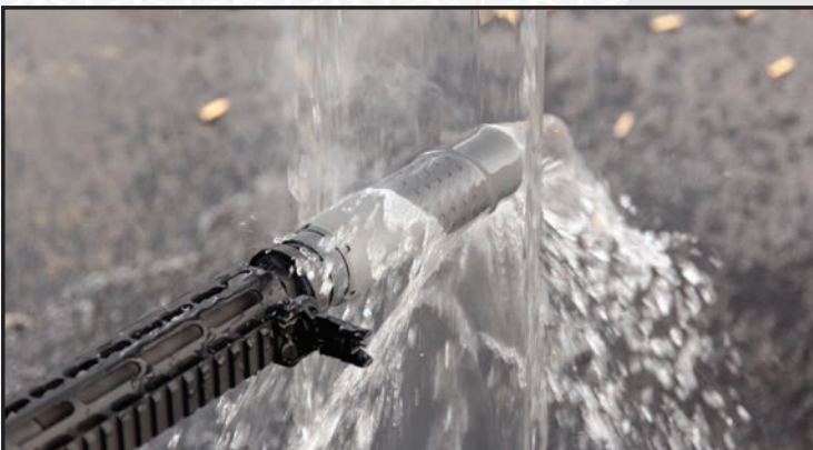
Suppressor being water quenched after 450 rounds in under 4 minutes.
